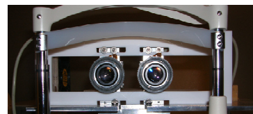
Figure 2. The binocular display system used to present the visual stimuli to the participants.
