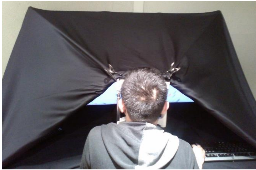
Figure 5.3 An illustration of a subject taking part in the experiment. Subjects will watch the stimulus with their head comfortably fixed on the chin rest. Black curtain was provided to mark off the irrelevant environment. Subjects could press the button to stop the stimulus at any time. Light were turned off during the experiment.
