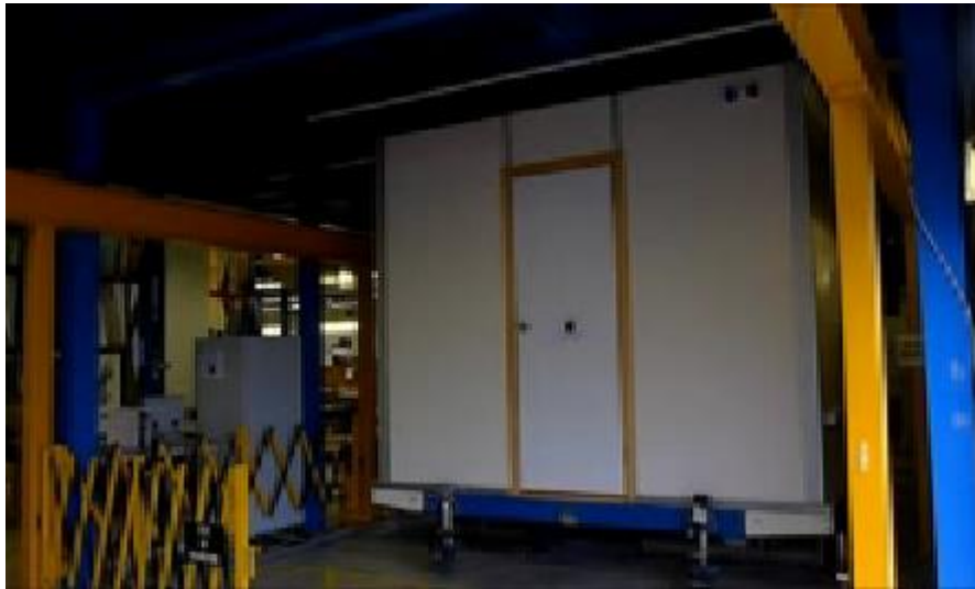
Figure B.1 A photo of the motion simulator used in the study. The motion simulator could move along the fore-and-aft axis (x) and lateral axis (y). It is designed and built in house at HKUST. The actuation is electromagnetic.
