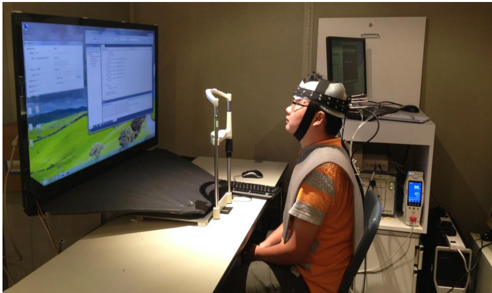
Figure 6.2 A photograph illustrating the experimental setup with the LCD screen, chin rest and the subject mounted with NIRS transmitters and detectors. A black curtain was temporarily removed for the photo taking.
