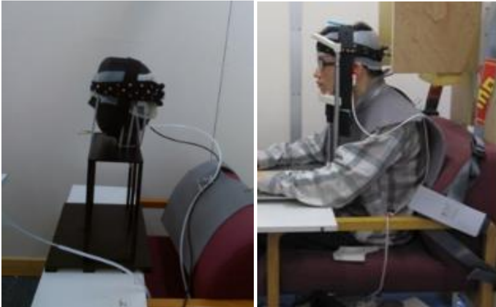
Figure 4.1 Photos of experiment set up in control experiment (study two) with a manikin and in experiment (study one) with human subject. As seen from the photo, we tried to replicate the set-up in the manikin experiment to be same with human subject experiment.
