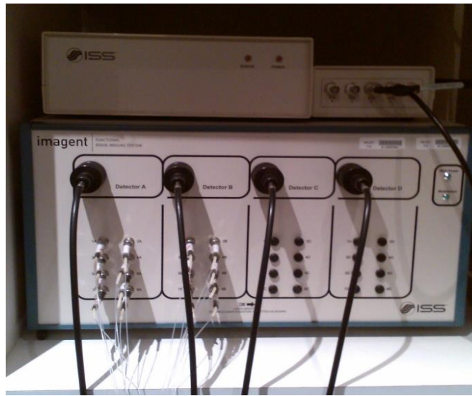
Figure A.1 Imagent ISS: near-infrared spectroscopy system. The Imagent ISS was adopted for NIRS measurement in all our experiments. The system has 4 NIR detectors and 8 pairs of NIR transmitters (one pair contains transmitters of two wavelengths).
