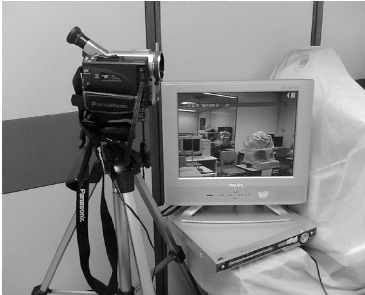
Figure 4.2: The monitor system for the main experiment. It consists of a camcorder and a DVD writer to record the experiment.
