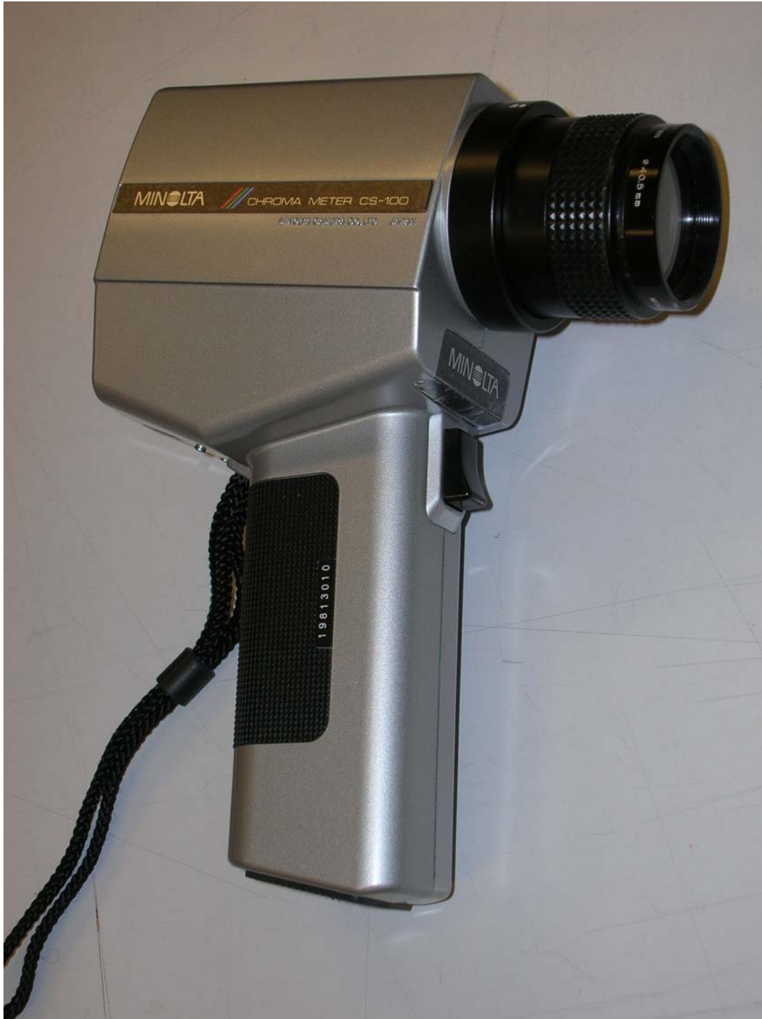
Figure 2.0 Chroma meter used for measuring the luminance of the microdisplay.
