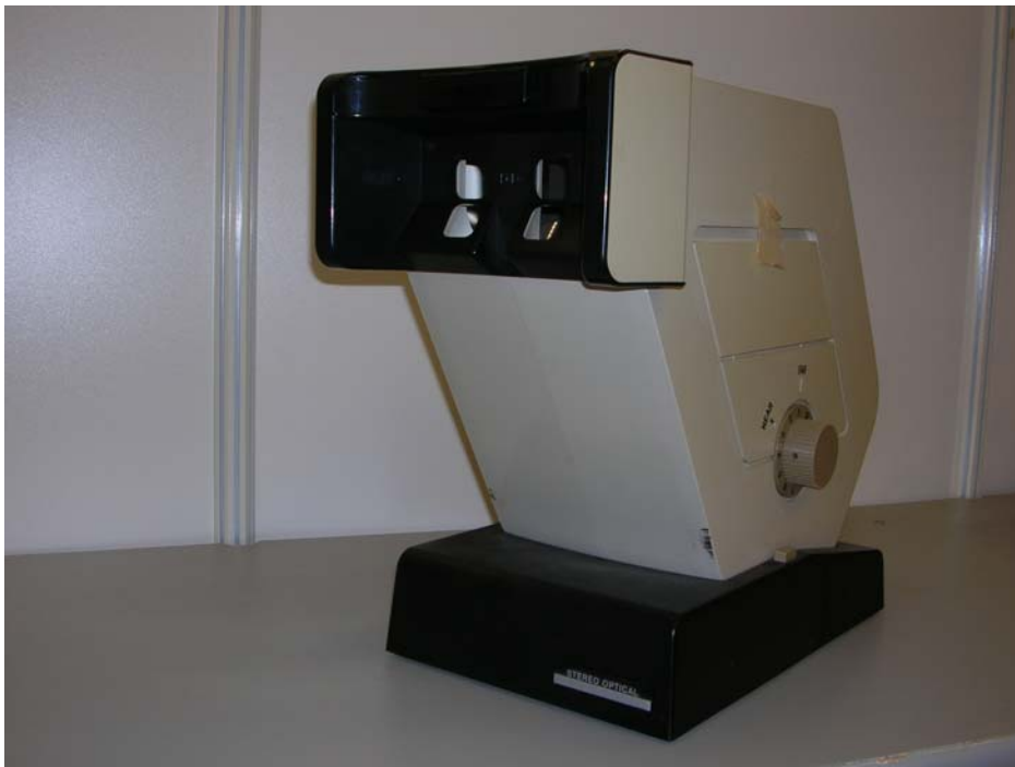
Figure C.1 Vision tester used for testing near and far visual acuities, stereoacuity and phoria of each subject. (Model: OPTEC 2000, made in U.S.A.)
