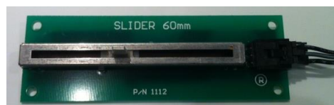
Figure 3.3 Hardware slider for user response
