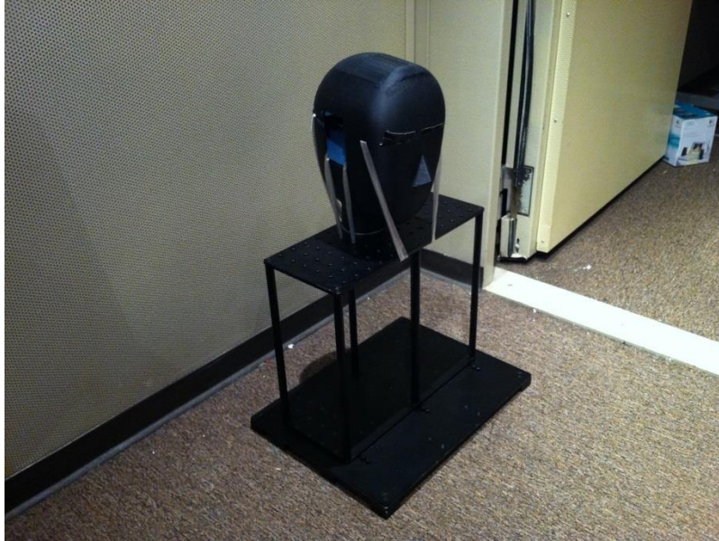
Figure 4.5a Mannequin head used for sound calibrations
