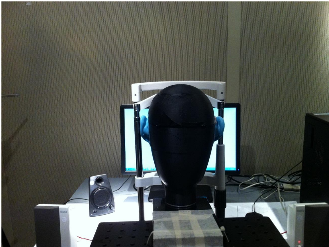
Figure 4.5b Silica pinna inserted in the mannequin head during sound calibrations
