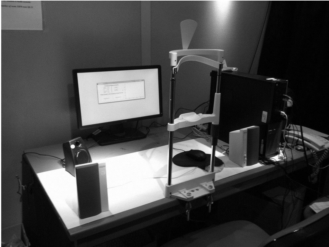
Figure 4.6 The experiment set-up inside the acoustic chamber. The speaker configuration for free-field presentation, the computer system for subject response and the chin rest are visible
