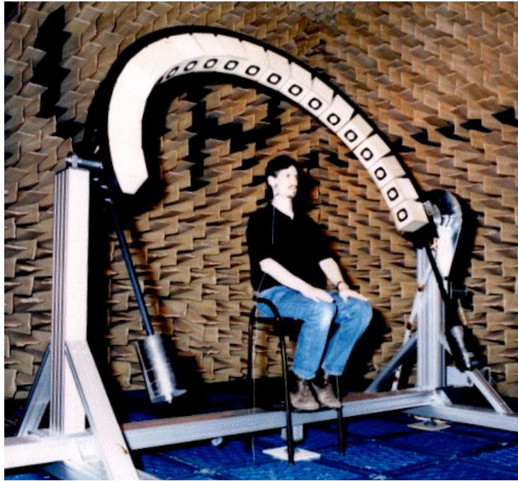
Figure 2: Localization measurement: Speaker array
