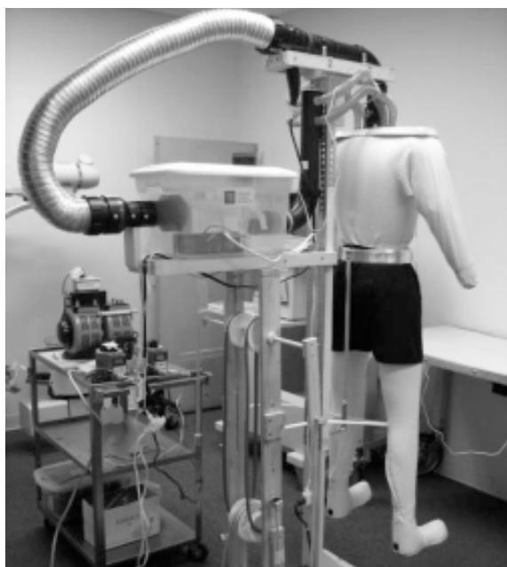
Figure 2. Inflatable thermal manikin used for assessing the effectiveness of the prototype reflective vests
